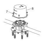
Secure protector(8) onto the base with screws(7).
